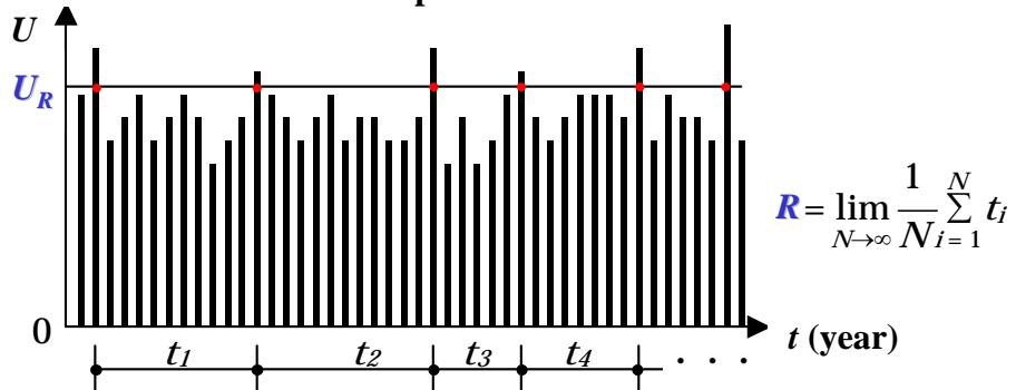
Return Period  $R$  = Mean Time Between Failure (MTBF)
