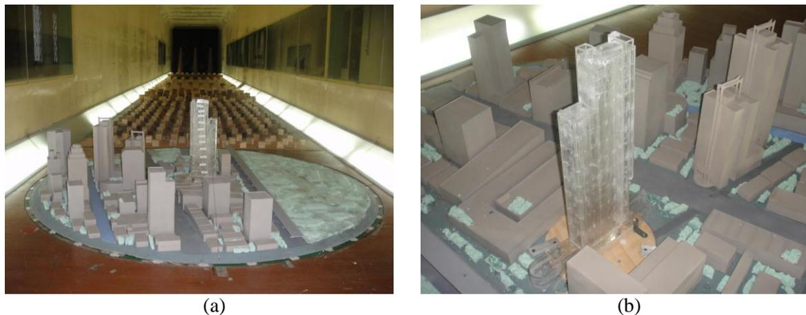
Figure 6. (a) Pressure measurement study of Circle II Building in Bangkok by wind tunnel test, and (b) Rigid model
