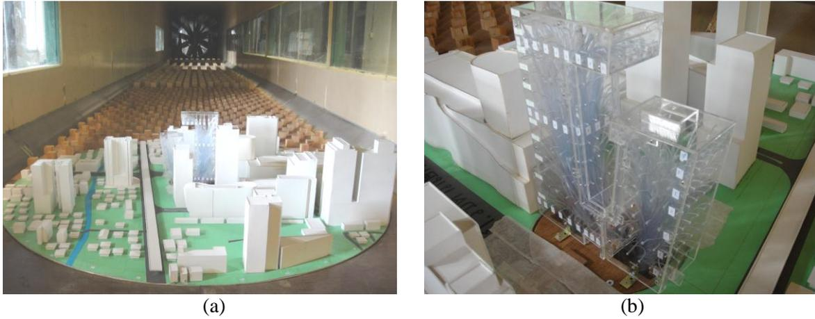
Figure 4. (a) Pressure measurement study of G Land Rama 9 building in Bangkok by wind tunnel test, and (b) Rigid model
