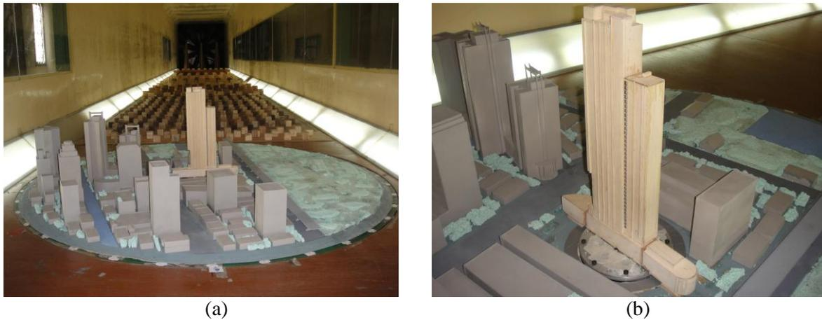
Figure 7. (a) Overall wind load study of circle II building in Bangkok by wind tunnel test, and (b) high-frequency force balance model
