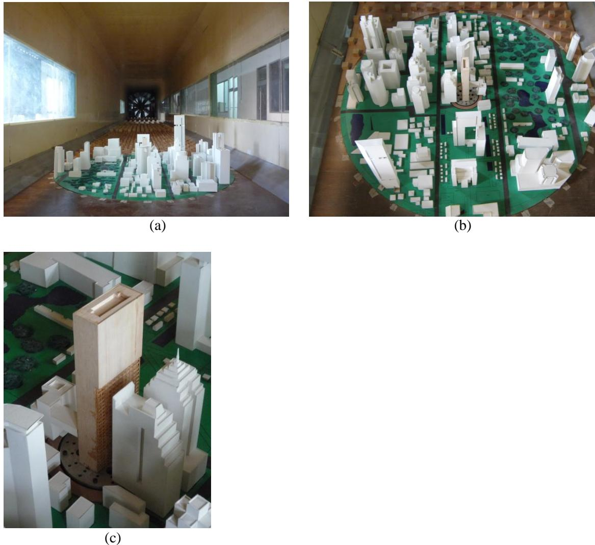
Figure 8. (a-b) Overall wind load study of Langsuan Block 3 building by wind tunnel test, and (c) high-frequency force balance model
