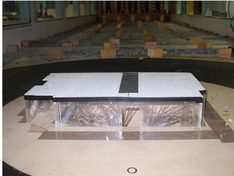
Figure 1: Model with a flexible Styrofoam roof inside the de Bray wind tunnel
