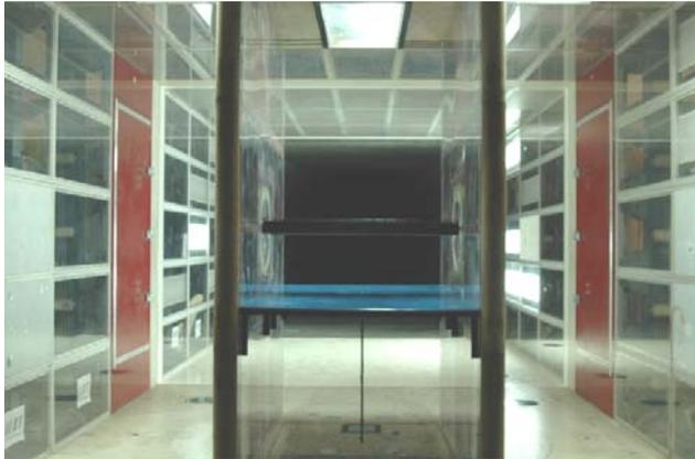
Figure 2. Installation of the Sectional Model in ILST Test Section
