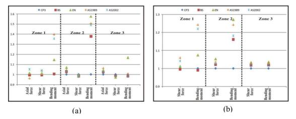
Figure 13: (a) Column loads (b) beam loads for load combination 1.0G+1.4W (wind flow perpendicular to 30m side)
