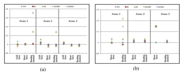
Figure 12: (a) Column loads (b) beam loads for load combination 1.2G+1.2Q+1.2W (wind flow perpendicular to 30m side
