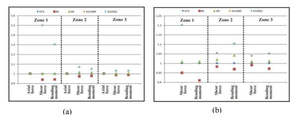
Figure 8: (a) Column loads (b) beam loads for load combination 1.2G+1.2Q+1.2W (wind flow perpendicular to 46 m side)
