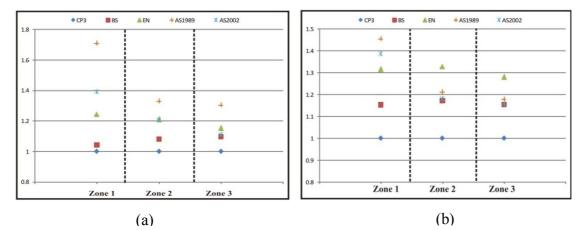
Figure 17: Maximum shell stress in shear wall of the 183m building (a) wind flow perpendicular to 46 m side (b) wind flow perpendicular to 30 m side
