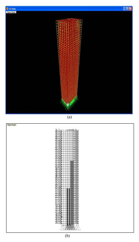
Figure 3: (a) Finite element 3 - D model of 183 m high building (b) Wind loads applied in windward and leeward side of the 183 m high building
