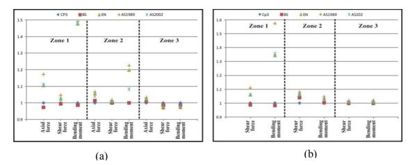
Figure 9: (a) Column loads (b) beam loads for load combination 1.0G+1.4W (wind flow perpendicular to 46 m side)
