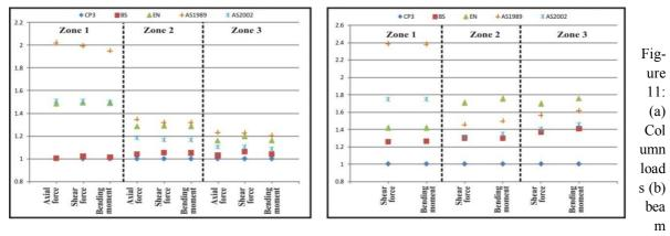
loads for wind load only (wind flow perpendicular to 60 m side)
