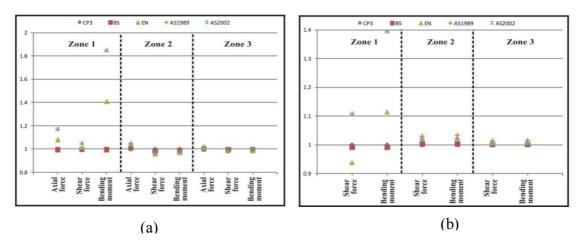
Figure 10: (a) Column loads (b) beam loads for load combination 1.4G+1.4W (wind flow perpendicular to 60 m side)
