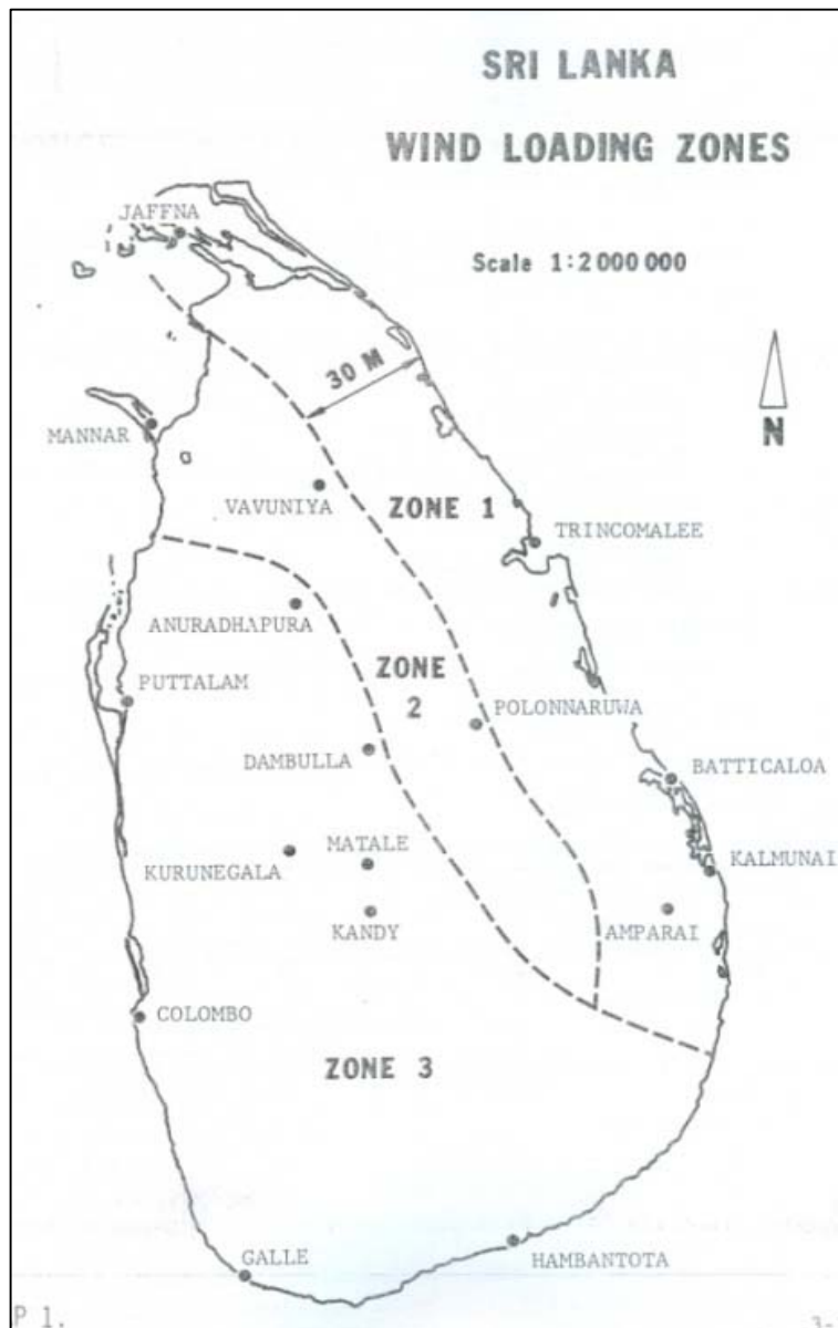
Figure 1: Wind Zones in Sri Lanka (Design manual “Design building for high winds”, 1978)
