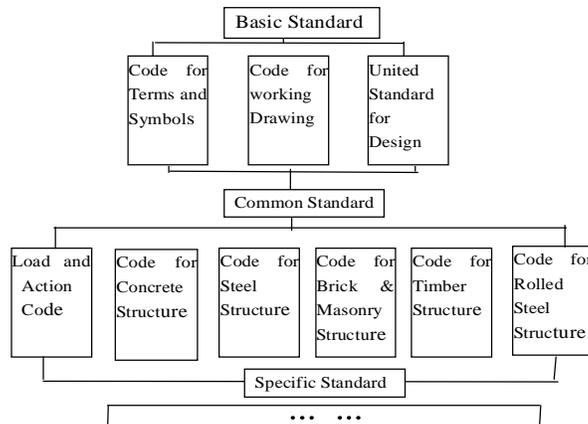
Fig. 3 The system of codes for design of building structures
