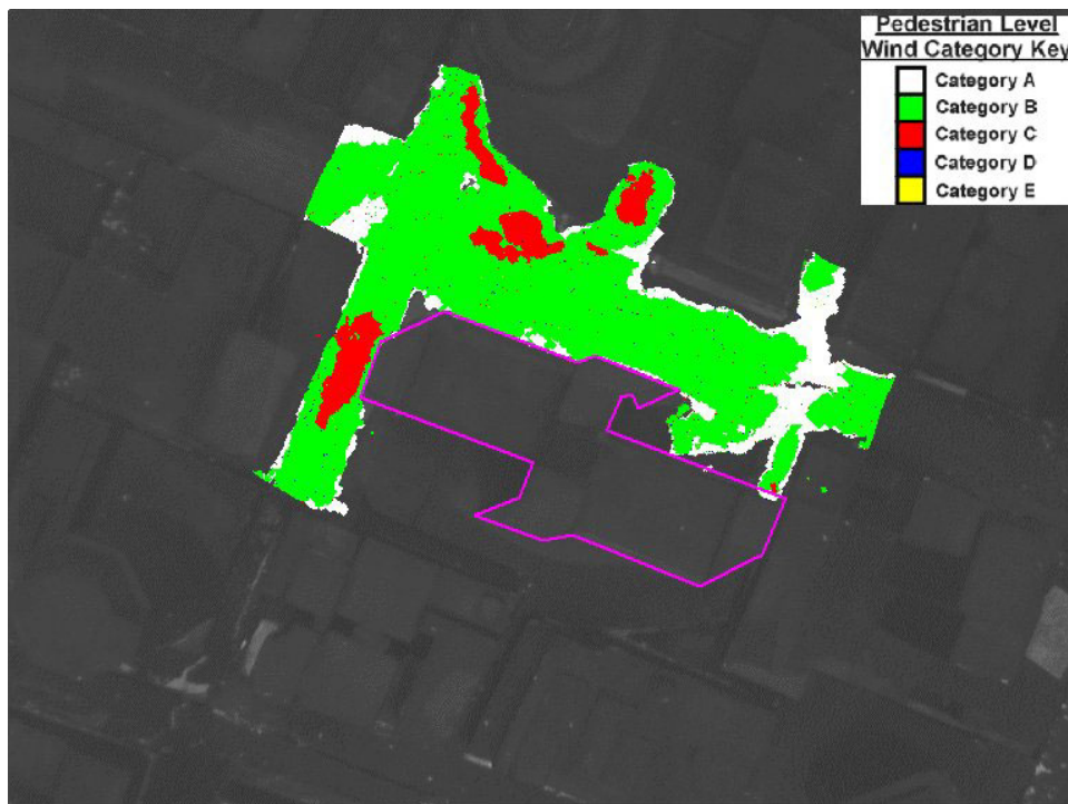
Figure 2. Wind categories in the vicinity of proposed modifications to a building in Auckland. (North is to the right of the figure.)
