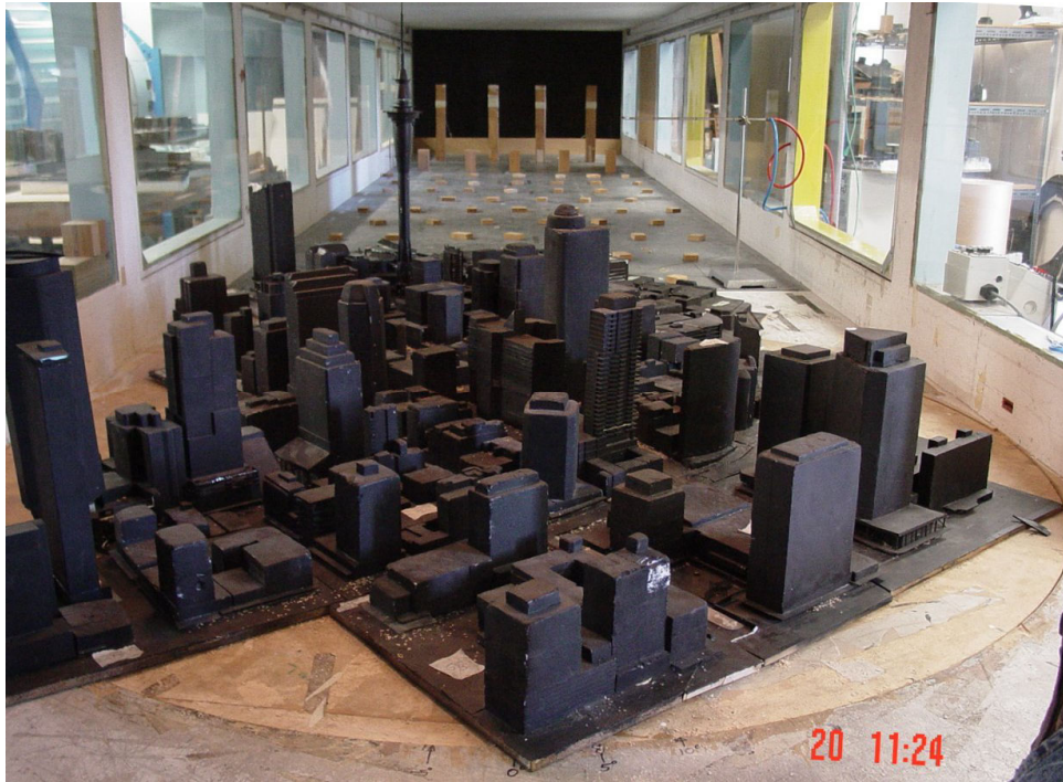
Figure 1. General view of the proposed development embedded in model of surroundings looking upstream (westwards) showing roughness blocks and trip barrier.
