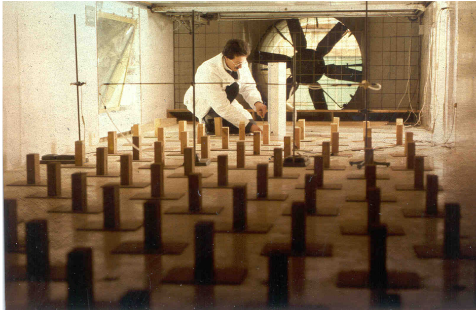
Figure 3. Photograph of the Central Laboratories wind tunnel looking downstream. There is a compliant "Parkinson-type" slotted roof over the turntable area.
