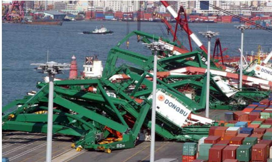
Fig. 2.1 Gantry Cranes Overturned by Typhoon Maemi
