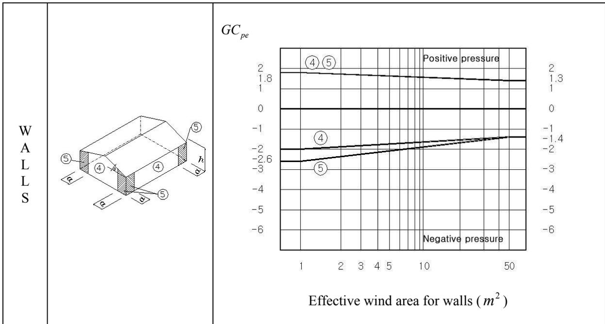
Notes: Each component shall be designed for maximum positive and negative pressures. 2) Vertical scale denotes  $GC_{pe}$  to be used with  $q_h$  based on terrain category C. 3) Values of  $GC_{pe}$  for walls shall be reduced by 10% when  $\theta \leq 10^\circ$ .
