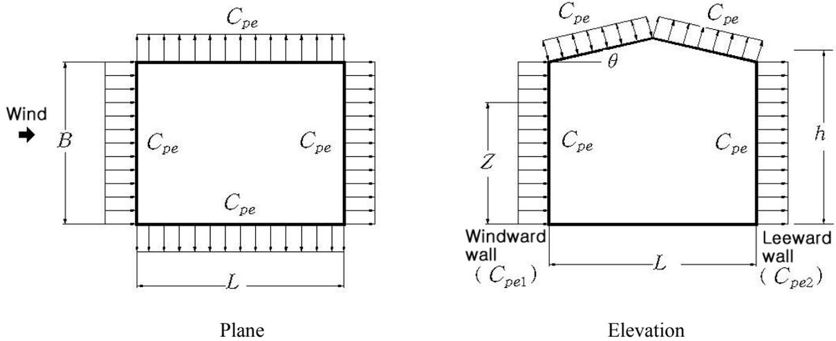
(a) External pressure coefficients for walls ( $C_{pe}$ )
