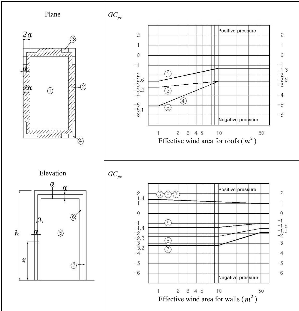
Notes: Each component shall be designed for maximum positive and negative pressures.
