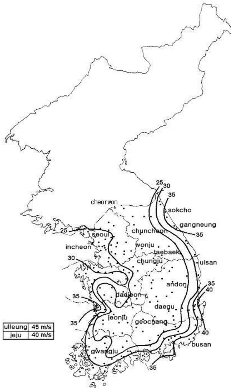
Figure 1 Basic wind speed  $V_0$  in Korea
