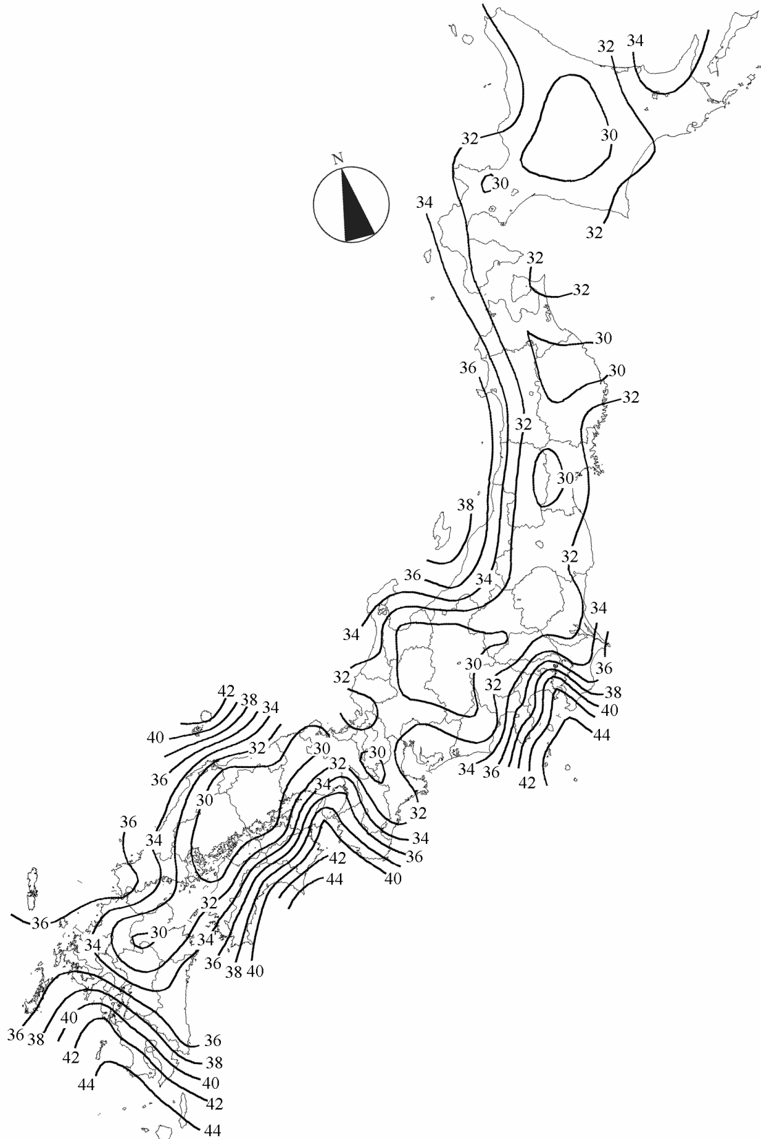
Figure 2 Basic wind speed specified in AIJ-RLB-2004 (100-year-recurrence)
