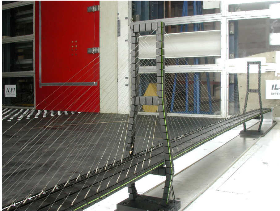
Figure 2. A long span bridge model in Indonesian Low Speed Tunnel (ILST)
